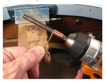
To wind a coil, just bend a right angle on the end of the wire about a half inch long and insert this into the screw gun chuck. Then wind slowly, keeping a tight coil. I like to rest the end of the mandrel on the edge of the table or bench pin. Finally, one note of caution. If you are winding an entire length of wire, be careful as you get near the end of the wire. If the end passes under your thumb, it can cause a nasty scratch or cut.
