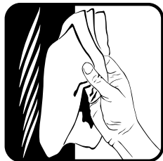
Degrease the surface
