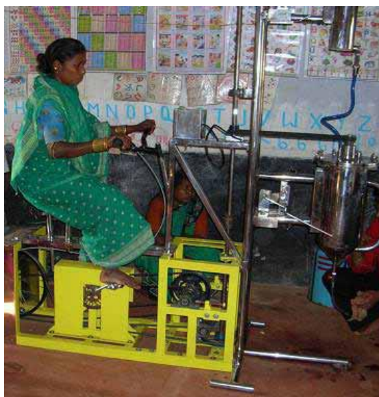
Fig. 2: Pedal-driven biodiesel reactor (Photo: CTxGreEn)
