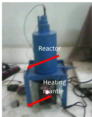
Figure 2: Batch Reactor used for the biodiesel conversion
