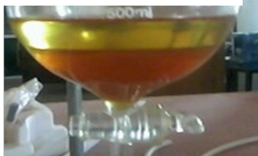
Figure 3: Phase separation of biodiesel and glycerine
