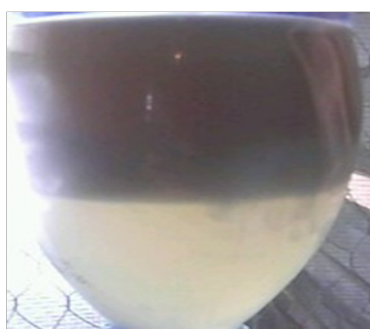
Figure 4: Phase separated of pure biodiesel and hydrated methanol
