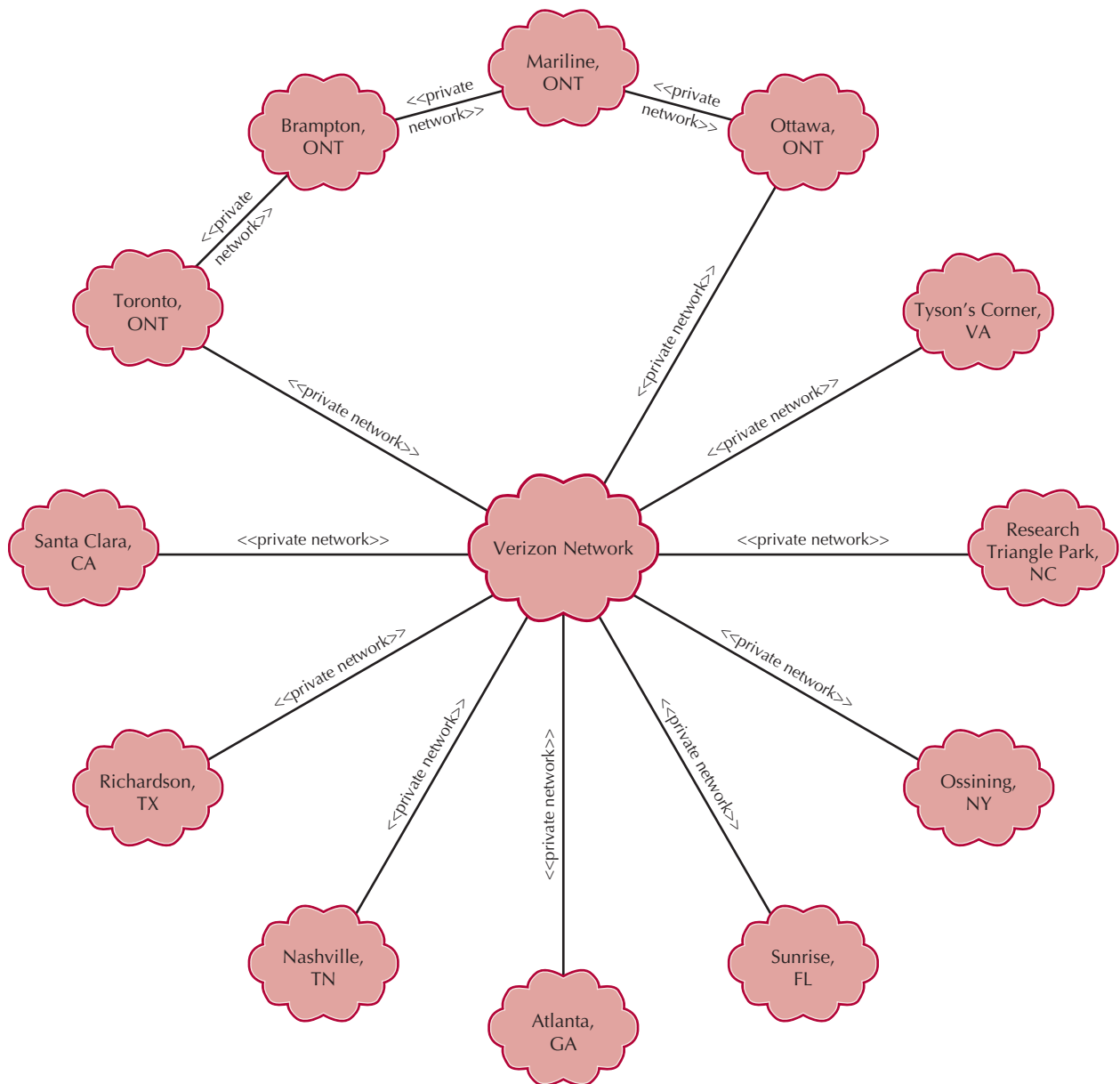
FIGURE 13-10 Deployment Diagram Representation of a Top-Level Network Model
