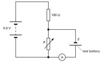
The supply battery may be assumed to have negligible internal resistance. The resistance R of the variable resistor is adjusted until R has a value of  $28 \Omega$  and the current shown by the ammeter is zero. Show that the e.m.f. of the test battery is about 1.1 V. [3]
