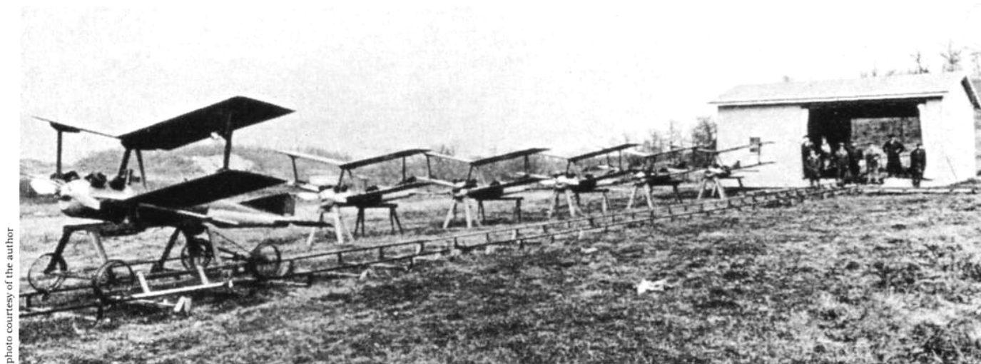
Buzz bombs were delivered in the form of a mini-biplane with 14-foot wingspan and Ford-designed V-4 aircraft engine.
