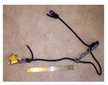
**Figure 2** An adjustable ascender that has been shortened for a shorter reach.
