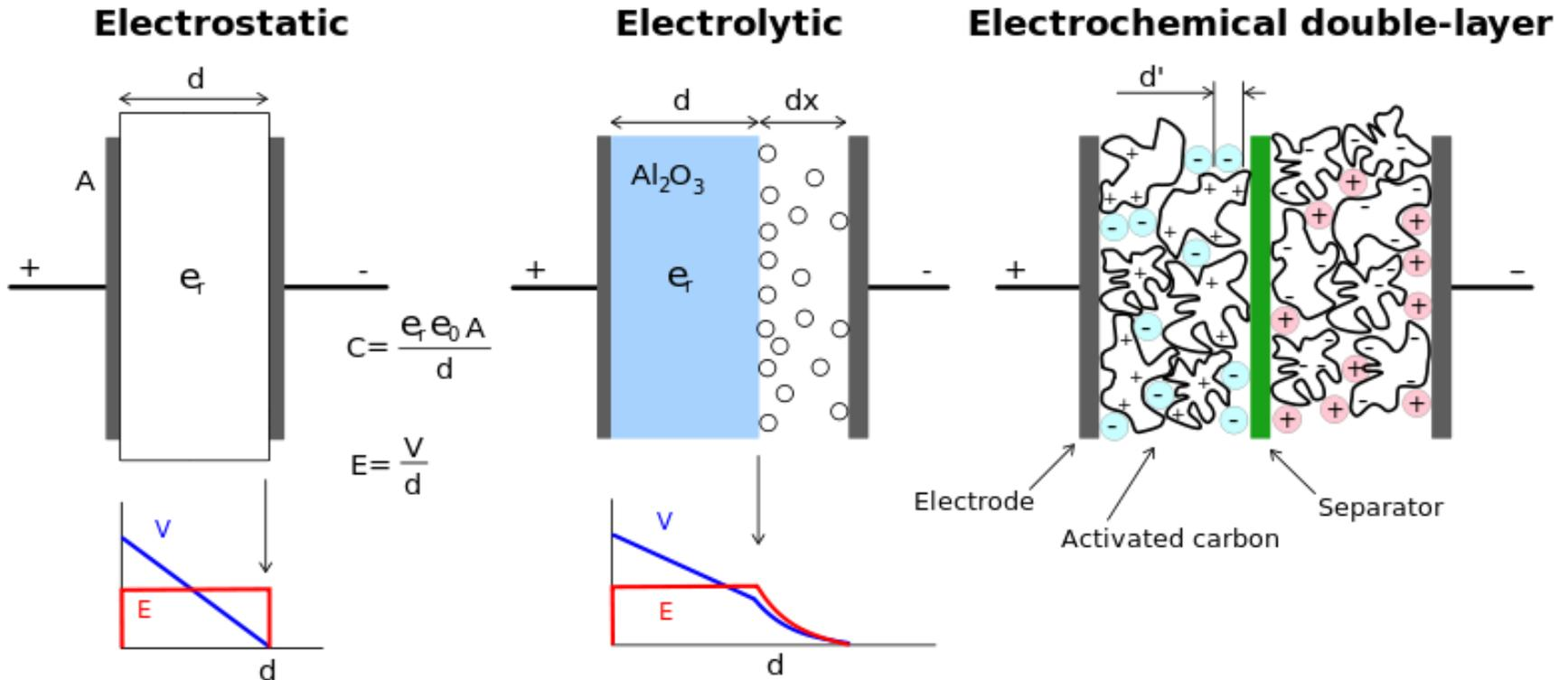
**comparison of construction diagrams of three capacitors.**
