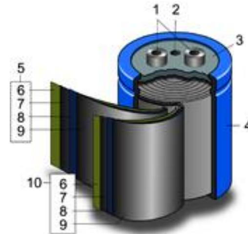
**Schematic construction of a wound super-capacitor**
