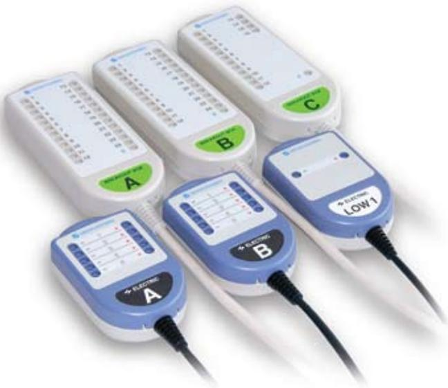
The Neuromaster utilizes small and compact breakout boxes for waveform acquisition and stimulation. These individual breakout pods can be placed either at the head or foot of the OR bed to help eliminate extensions or long electrode wires.
