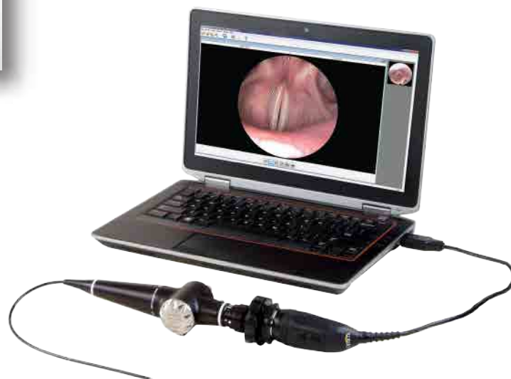
Optim's ENTity LED Nasopharyngoscope is seen coupled to the VidCap Camera System and then connected to a standard laptop for easy image viewing.
