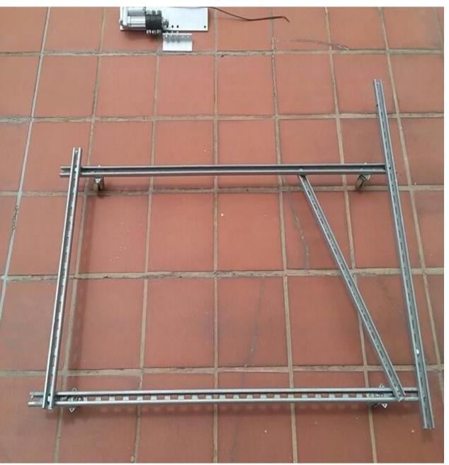
The manifold brackets are premounted onto U-shaped fixing rails of dim. 28x19 mm and tightened to the rail with square plate-nuts M8.
