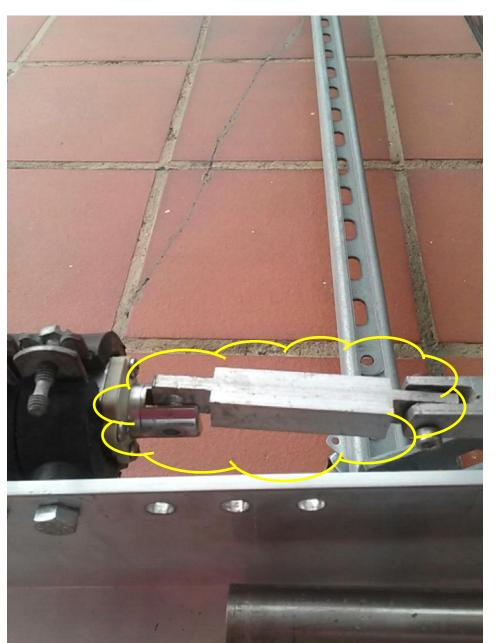
Place the flap mechanism connector in line with the closed linear motor connector.
