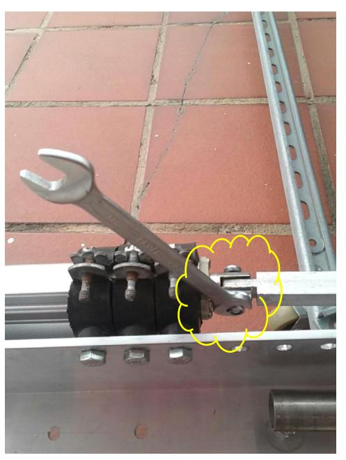
Put on the 6 mm locking nut and tighten securely with a 10 mm key
