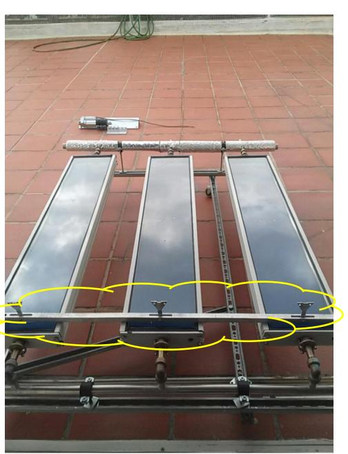
Bring the flap tilting mechanism into place positioning the connector towards the motor position.
