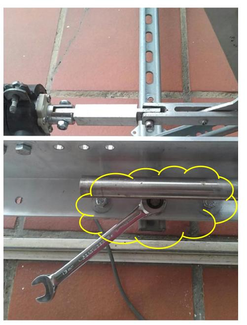
Straighten up the fixture to be in line with the U-shaped rail and tighten the three 8 mm screws with a 13 mm key
