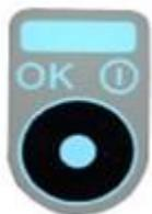
Switches the programming mode, confirms the settings, and turns the unit on or off (hold for 3 seconds).
