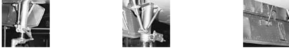
• Image 16: The nose gear well and door are painted aluminum.
