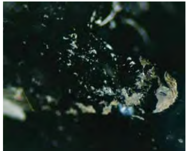
Figure 32. In the heat-treated tourmalines, the larger cavities in partially healed fissures often appeared somewhat frosty, which indicates that the fluid dried out during the heating process. Photomicrograph by J. C. Zwaan; magnified 40 \times .
