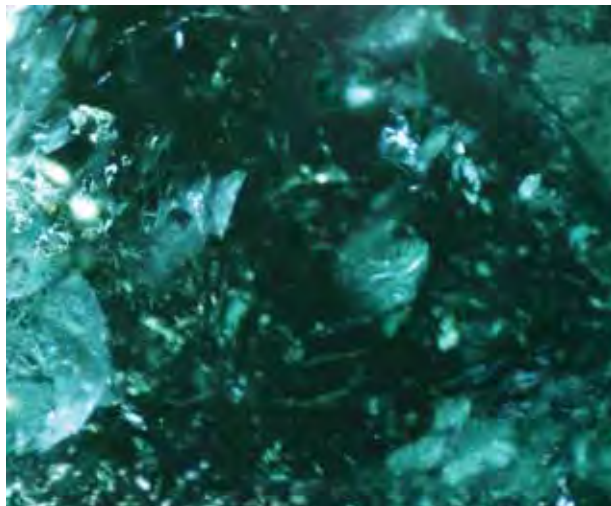
Figure 31. Minute and slightly larger cracks were common in most of the heated tourmalines, showing both discoid and more elongated shapes. When viewed with darkfield illumination, they often appear as milky stress fractures or otherwise translucent areas. Photomicrograph by J. C. Zwaan; magnified 16 \times .
