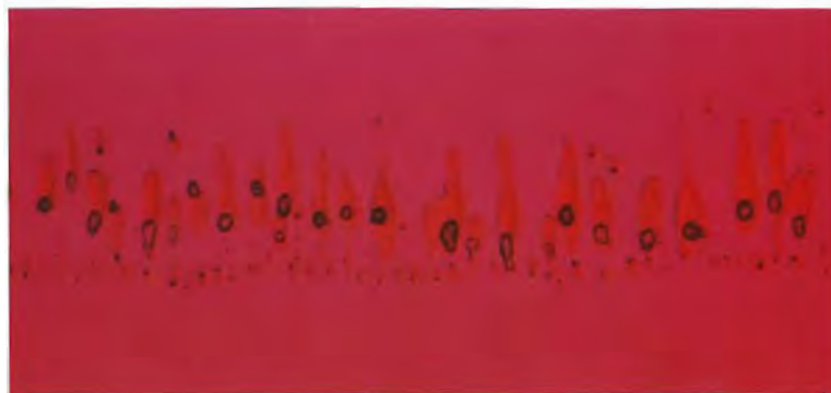
Figure 19. These small flux inclusions, in parallel alignment, are transparent. Note that each contains a prominent bubble, which appears in high relief against the flux. The flux itself shows low relief against the ruby, which indicates that its refractive index is close to that of the ruby. Magnified 50 \times .
