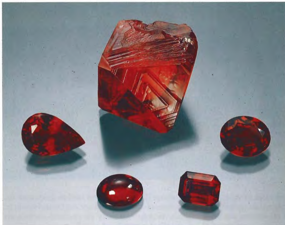
Figure 1. This 44.74-ct rhombohedral crystal and the accompanying cut stones (from left to right—4.93, 2.55, 2.14, and 3.51 ct) are representative of some of the Douros flux-grown synthetic rubies that have been produced to date. Samples courtesy of John Douros, Piraeus, Greece; photo by Robert Weldon.
