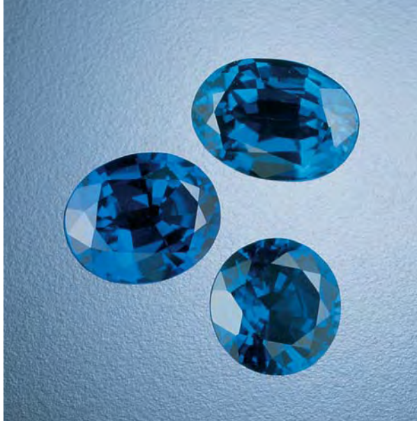
Figure 8. Tairus researchers produced these greenish blue hydrothermal synthetic sapphires by doping them with \text{Ni}^{2+} and \text{Ni}^{3+} and, in some cases, \text{Cr}^{3+} . Photo © GIA and Tino Hammid.
