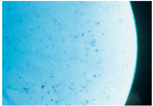
Figure 13. Flake-like crystalline inclusions are abundant in many of the green-to-blue Tairus hydrothermal synthetic sapphires. Photomicrograph taken by S. Z. Smirnov, with sample between crossed polarizers, immersed in methylene iodide, magnified 25 \times .
