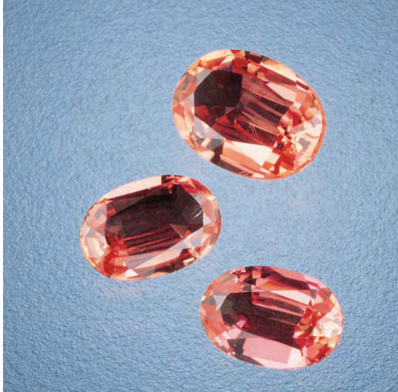
Figure 9. The colors of these pinkish orange "padparadscha" ( \text{Ni}^{3+} - \text{Cr}^{3+} ) Tairus hydrothermal synthetic sapphires are similar to those seen in nature or in other synthetic sapphires. Photo © GIA and Tino Hammid.
