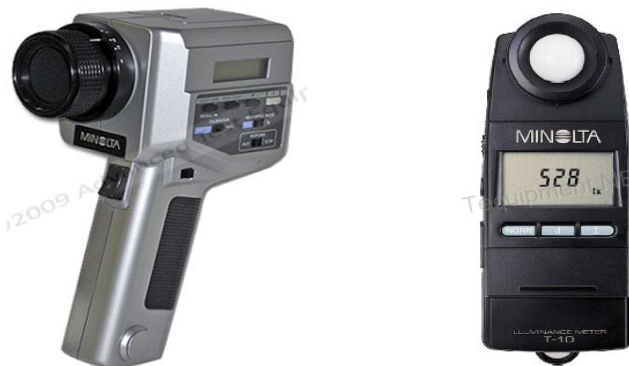
Figure 5. a. Minolta LS-100 Luminance Meter; b. Minolta T-10 Illuminance Meter.
