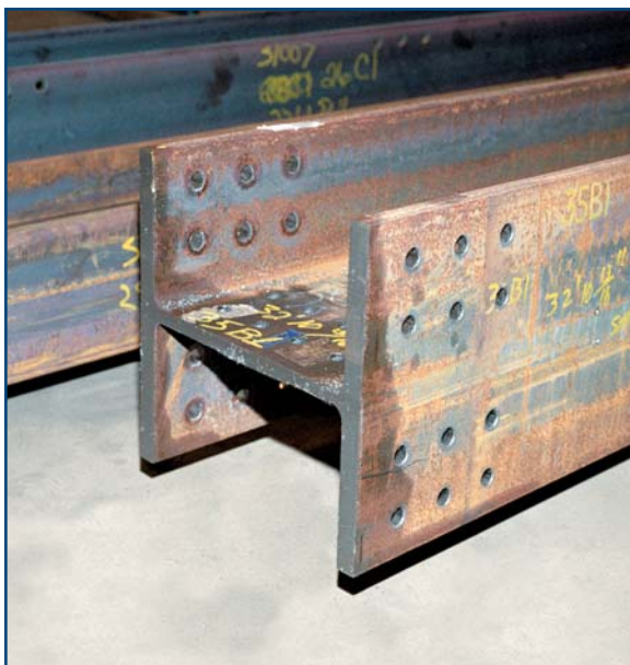
Cutting and Drilling
