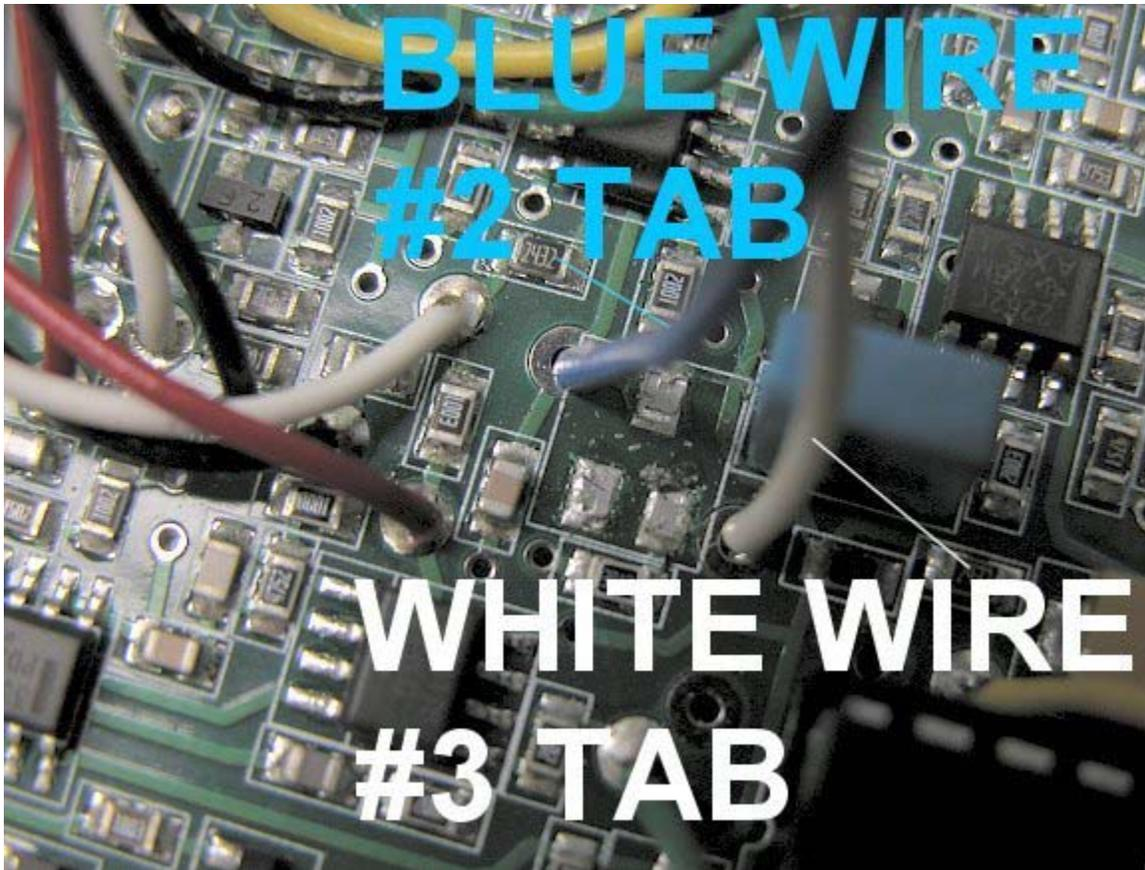
You will notice there are 3 contacts on the orig. trim pot as well as on the external Bourns pot you will be using. Tesoro only uses two of the pots contacts. You may ask why there 3 trimmer contacts soldered to the circuit board? Two are being used, the third was just soldered to a dummy pad that provides no function.
