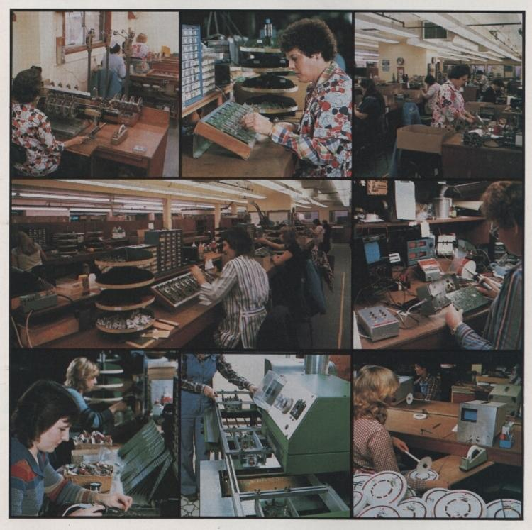
Many of White's parts are created especially for their mineral/metal detectors. Only the finest components, carefully tested before and after insertion into a unit, will meet White's strict standards for quality and performance. Each detector is built by precision craftsmen and technicians. The strong metal boxes are formed at White's Sweet Home factory. Cir-
