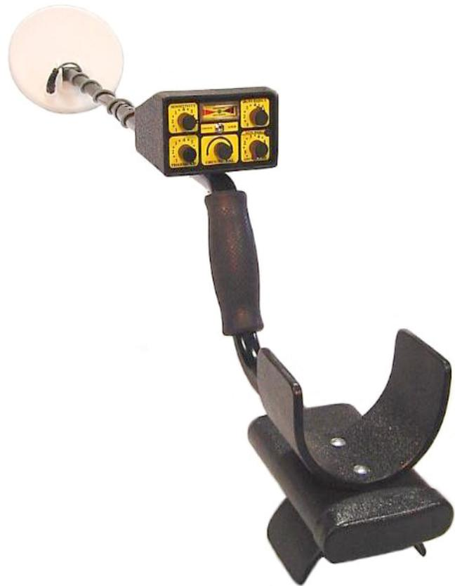
The depth of the Ground Hawk depends on the target, mineral content, and the water content in the soil. The wetter the soil is, the greater the depth. The Ground Hawk has a built in speaker, it also has a headphone jack. The detector contains 8 AA batteries, which is included in your purchase.
