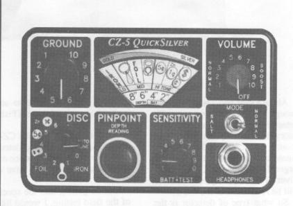
Fisher's CZ-5 QuickSilver control panel showing the target ID system's unique design.
