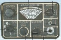
Pushbutton, no-motion pinpoint control also gives depth reading
