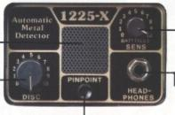
Push button activates all-metal, zero-motion, pinpoint mode Dual-purpose potentiometer with switch controls sensitivity and battery check
