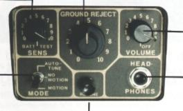
Adjust target volume and turn power on/off
