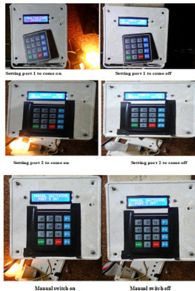
Fig. 14: Output Ports timing control test.
