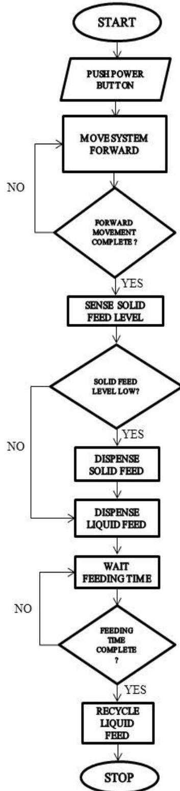
Figure 7: Mobile Intelligent Poultry Feed Dispensing System Flowchart
