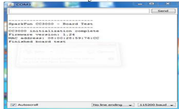
Figure 13 Board test of the CC3000 wifi shield
