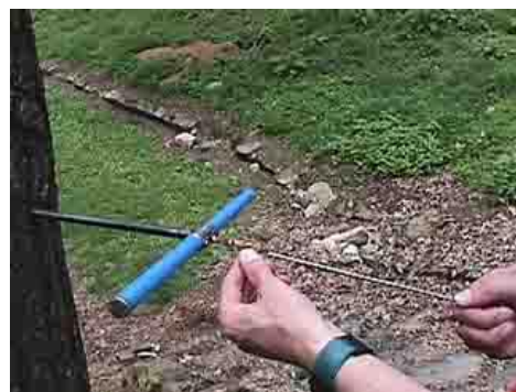
Fig. 10.9 The core extractor is inserted into the hollow increment borer.
