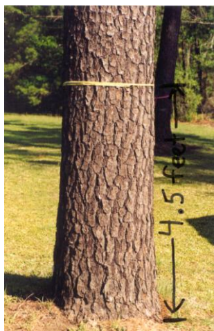
Fig. 10.1. Diameter is measured 4.5 feet above ground.
