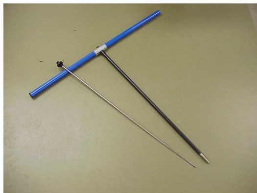
Fig. 10.7 Increment borer (blue handle with hollow, threaded bit).
