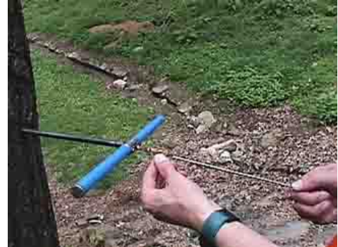
Fig. 10.9 The core extractor is inserted into the hollow increment borer.
