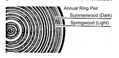
Figure 4.3. Annual rings consist of two separate rings — a light ring and a dark ring, grown each year.
