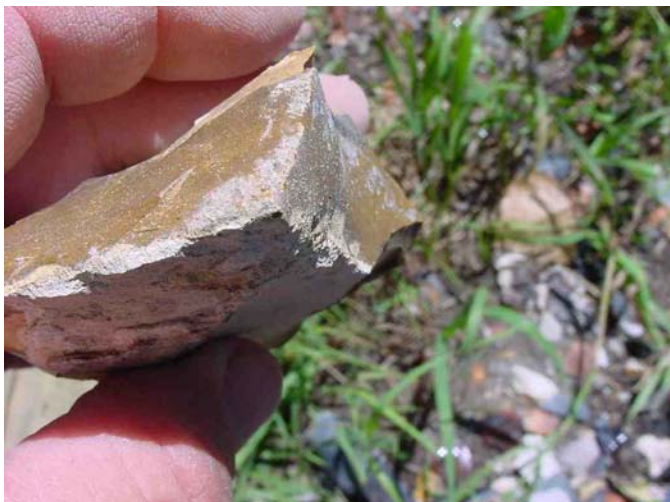
A tabular piece of Republican River material a.k.a. Republican, Niobrarite, Smokey Hill Jasper, Smokey Hill Silicified Chalkstone. The piece is approx. 2 1/2" wide, 4" long, and 1 1/2" thick. The piece is triangular in cross section
