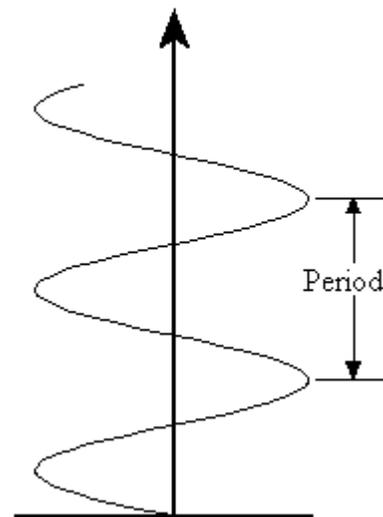
**Period** -- The time (usually measured in seconds) to complete one cycle of a vibrating system. The period is the reciprocal of the system's frequency.
