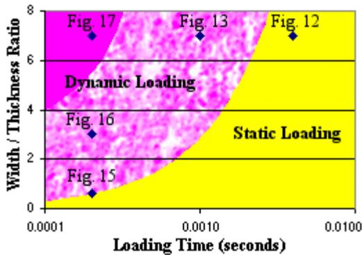
**Figure 14** -- The loading regions of a 3" wide biface. The yellow is the static mode region and the purple is the dynamic mode region. The dynamic region is further subdivided into lighter purple and darker purple. In the yellow and lighter purple regions all the flake types except the hinge flake can be created. The darker purple is the region of hinge flakes caused by the second harmonic in the core's vibration.
