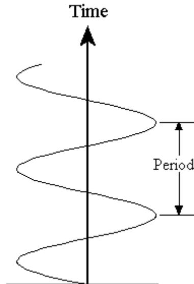
**Cycle** -- The motion that repeats itself in a vibrating system. A cycle is the vibration during the period.
