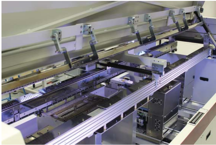
Fusion 4 (flux / top and bottom I.R. pre-heat / solder / solder)
