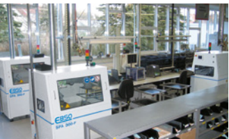
Production at Werma Signal Lights in Germany: 3 SPA machines, inbetween operator working place insures highest flexibiliy and throughput - always 3 different (or same) products are in production at the same time
