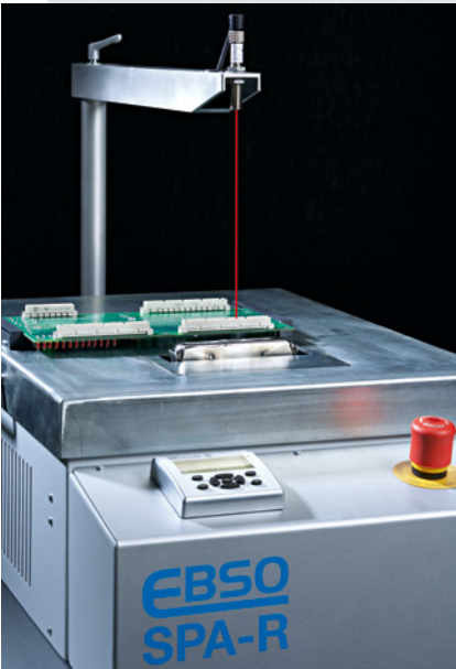
SPA-R with laserpointer to ease component centering over nozzle
