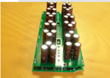
Selective soldering application with 45 mm interfering edge
