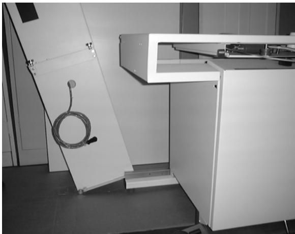
**Figure 5 – Mounting Tubestand on Rail**
