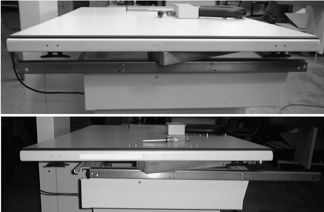
**Figure 7 – Table Top Raised; Bearing Track Moved Forward For Mounting Tubestand**
