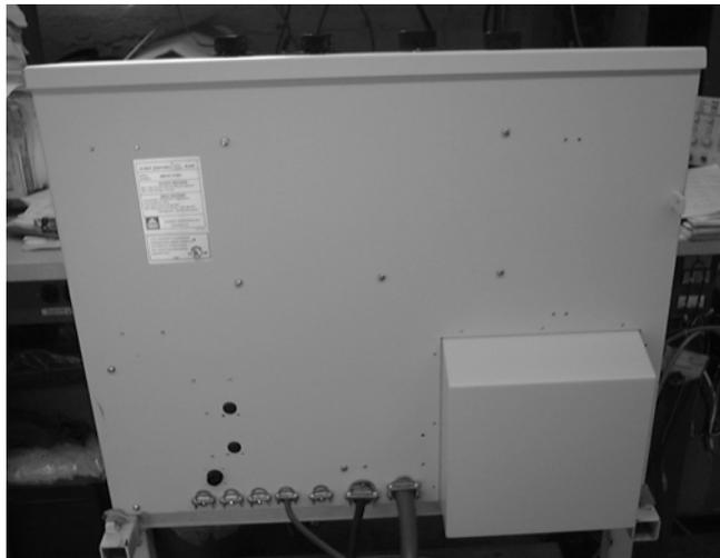
**Figure 13 – Rear of Control Showing Cable Entry Points**
