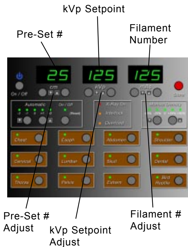
Figure 5-2c VET APR Operator's Console Calibration Configuration
