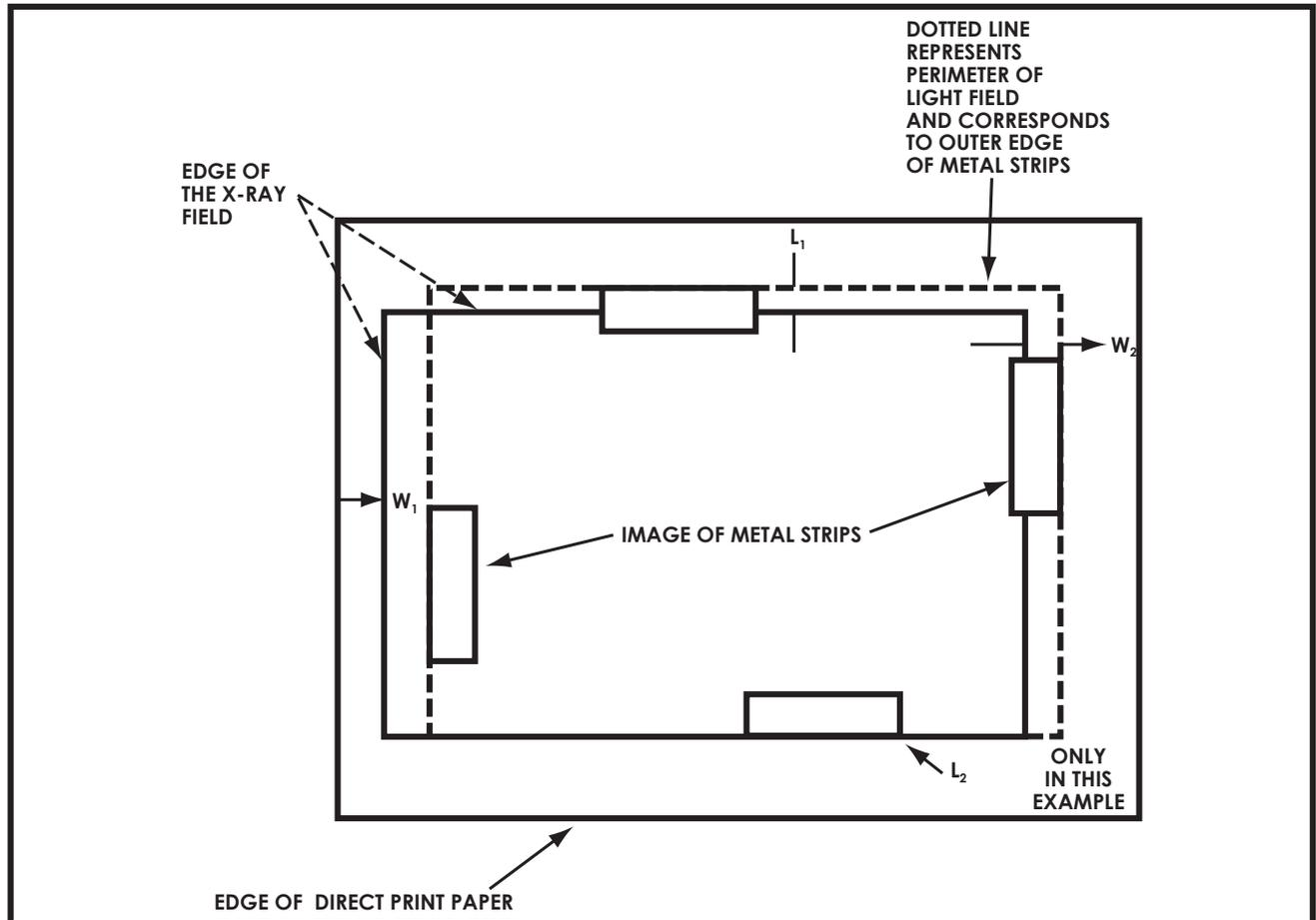
FIGURE 5.3 LIGHT FIELD vs. X-RAY FIELD ERROR MEASUREMENTS
