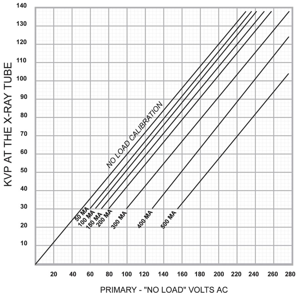
Plot of KVP Curve for TXR 325-1 and TXR 625-1 High Voltage Generator with the TXR 325D, TXR 325M, TXR 425 and TXR 525 SFQ X-ray Control.
