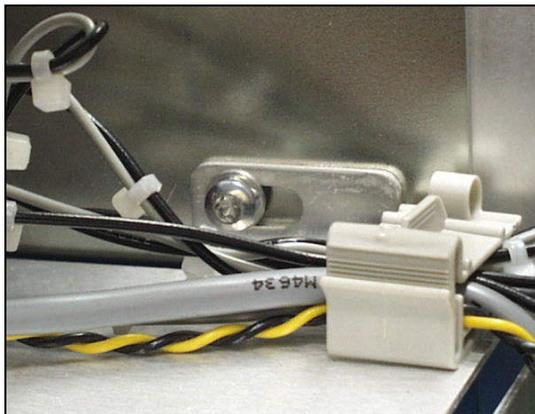
**Capacitor/Power Module Mounting Screw**
