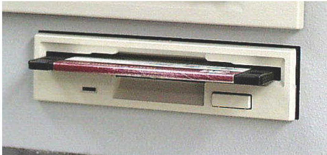
**3.5-Inch, 1.44-Megabyte Floppy Disk Drive on Workstation Rear Panel**
