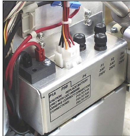
**Capacitor/Power Module Connectors**
