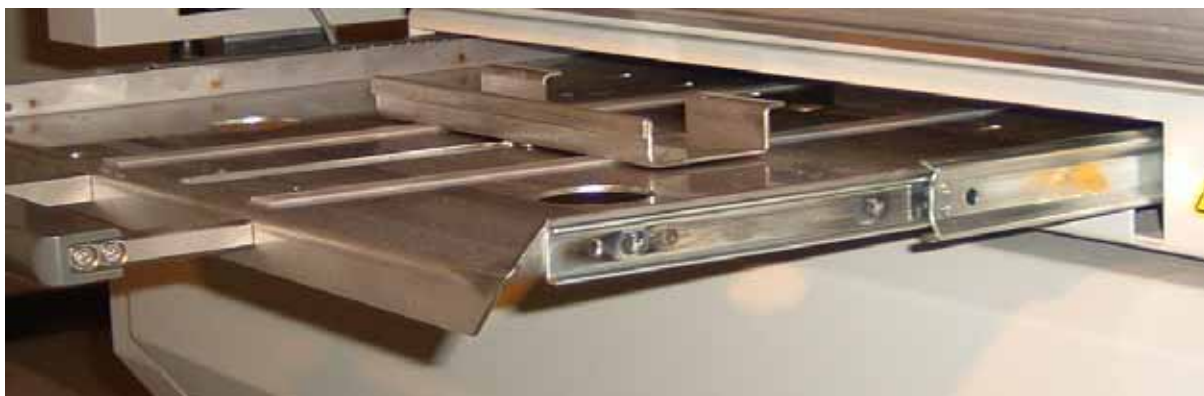
The cassette tray is supported in a telescopic roller guide
