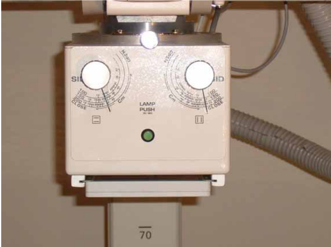
Collimator with dose area product measurement chamber
