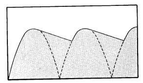
CABLE CAPACITY AT LOW MA changes the wave-shape of the energy reaching the X-ray tube from that shown by the dotted lines to a near constant potential form. The actual shape depends on cable length, kVp, and mA.
