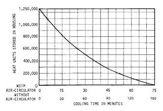
and since in this case the heat units per exposure is 7,200, therefore two exposures per minute  $(2 \times 7,200 = 14,400 \text{ units})$  could be made safely.
