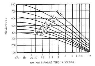
To illustrate, assume a technique of  $100~\rm{kVp}$ ,  $400~\rm{mA}$ ,  $1/10~\rm{second}$ , at the rate of 6 exposures per second for a total time of 3 seconds; using a tube having the above radiographic rating chart.
