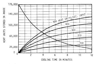
Solution: Refer to the anode cooling curve for the tube (above) and note that  $100,000 \, \text{HU}$  is at a cooling time of  $2-1/2 \, \text{minutes}$ .
