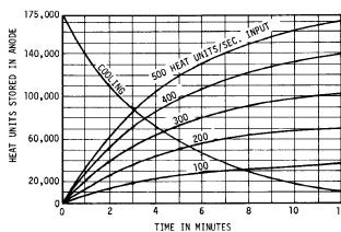
Use to determine permissible fluoroscopy and spotfilm exposure schedules.\*
