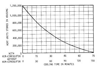
and since in this case the heat units per exposure is 7,200, therefore two exposures per minute  $(2 \times 7,200 = 14,400 \text{ units})$  could be made safely.
