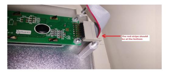
Make sure to plug the flat cable from the switch panel into this p.c. board, the ribbon cable into it's connector and the red and black wire into it's connector for the backlight, into this board.
