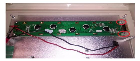
The ribbon cable can plug in the correct direction and the wrong direction. If it's plugged in the wrong way it normally does not damage anything, you just won't have a working display.
