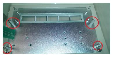
The nylon nuts are provided for the display so that circuit of the display is not shorted on the right side. On some older displays this was a problem.
