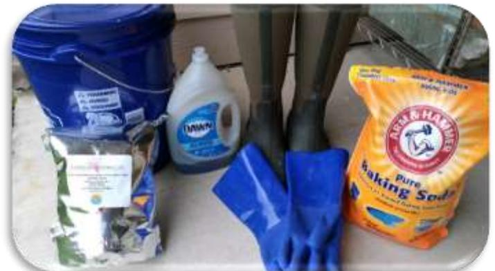
and added one cup of acid to the bucket, gently stirred the water and acid until the acid was dissolved – a broom handle works well for this. Important safety note here – always add acid to water not water to acid, so you don't splash any acid water on you. If you do get splashed, flushing with lots of running water and baking soda will neutralize the acid. Seek medical help if you get any acid in your eyes, nose, mouth etc.
