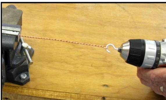
Note that a power drill is too fast a tool for this unless you have one with variable speed.
