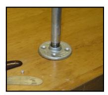
**FOREDOM STAND**—A quick and easy way to suspend a flex shaft over your jewelry bench is to use some steel pipe components from your local hardware store. It attaches with a couple screws and only costs about \$10.
