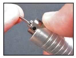
So I have two ways to speed up that task. For opening up the jaws, I just remember "four", the number of turns I have to make to open the chuck just enough from the 3/32 bur shaft size to the larger 1/8 bur shaft size.
