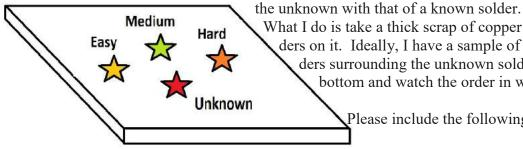
What I do is take a thick scrap of copper or nickel and arrange several solders on it. Ideally, I have a sample of easy, medium and hard known solders surrounding the unknown solder. Then I heat the plate from the bottom and watch the order in which the solders melt.
