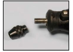
A simple and inexpensive (\$12) adjustable chuck solves all of this. It's available in most large local hardware stores or model-making outlets. Tightening the chuck is done easily by hand to any size shaft. No key is required.
