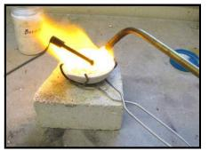
The procedure is straightforward. Heat the new melting dish to red with a large torch. You'll need plenty of heat. I use an acetylene/air Prest-O-Lite torch with a large #5 nozzle.
