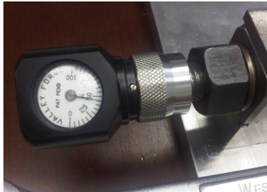
Gauge that easily snaps on and off SPC4™ bolt end for accurate load readings
