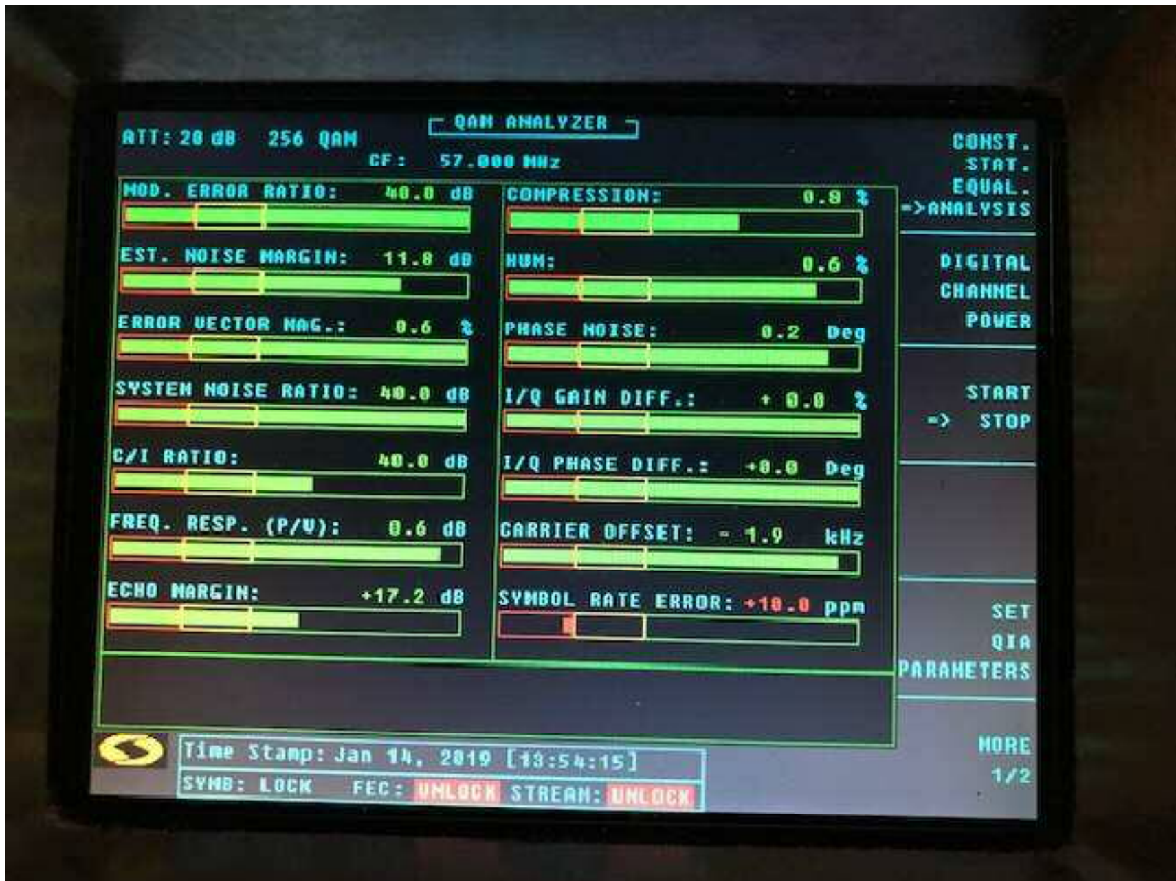
QAM Impairment Test on Channel 2. Symbol Rate Error failure is due to a known firmware 'bug' that was not fully resolved until version 4 hardware. Symbol Rate Error is not required by SCTE 40 specifications so this does not present a problem for full FCC POP testing compliance.
