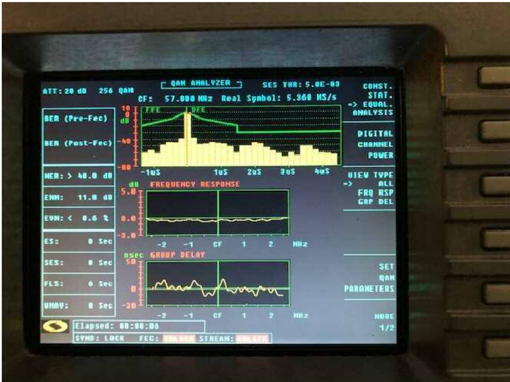
QAM analysis including adaptive equalizer activity, in-channel response, and group delay of Channel 2 test carrier.
