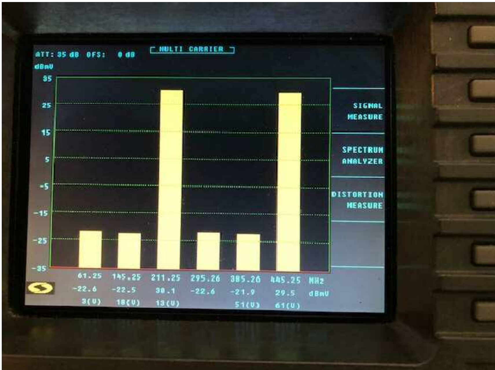
Multi Carrier mode with only channels 13 and 61 activated in my lab.
